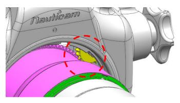
1. The SFE1224-Z zoom gear can be controlled by zoom/focus knob of the housing.
