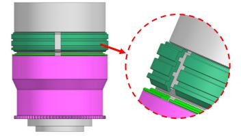
3. Insert the plastic C-ring for focus gear as shown and place it over the lens
