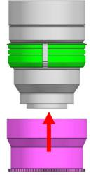
2. Insert the SFE1224-Z-Zoom gear on the plastic C-ring until it reaches the flange of the plastic C-ring.
