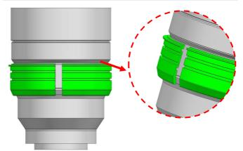
1. Insert the plastic C-ring for zoom gear as shown and place it over the lens
