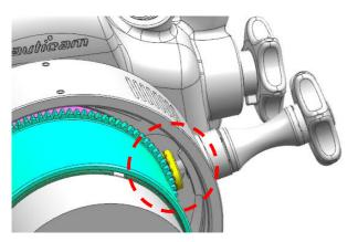
2. The SFE1224-F Focus gear can be controlled through the focus knob of #37305 N100 to N120 35.5mm Port Adaptor II
